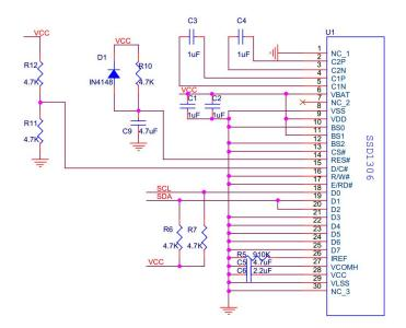
The I2C communication interface consists of slave address bit DC, I2C-bus data signal SDA (SDAOUT/D2 for output and SDAIN/D1 for input) and I2C-bus clock signal SCL (D0). Both the data and clock signals must be connected to pull-up resistors.
